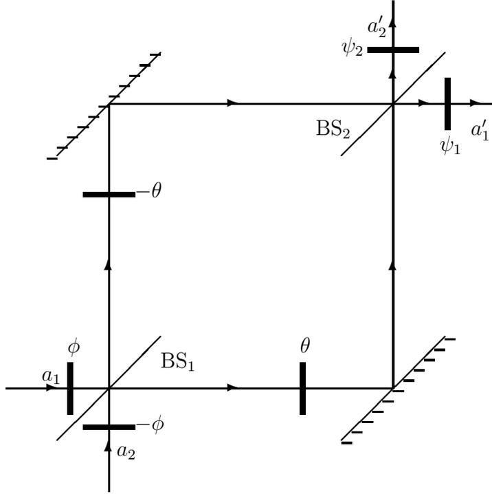
FIG. 2. Mach-Zehnder Interferometer implementing arbitrary  $U(2)$  transformation on two modes at the same frequency but differing in their direction of propagation.  $BS_1$  and  $BS_2$  are 50:50 beam splitters and thick lines are phase shifters by angles indicated.  $a_1, a_2$  are the annihilation operators at the input port and  $a'_1, a'_2$  are the annihilation operators at the output port
