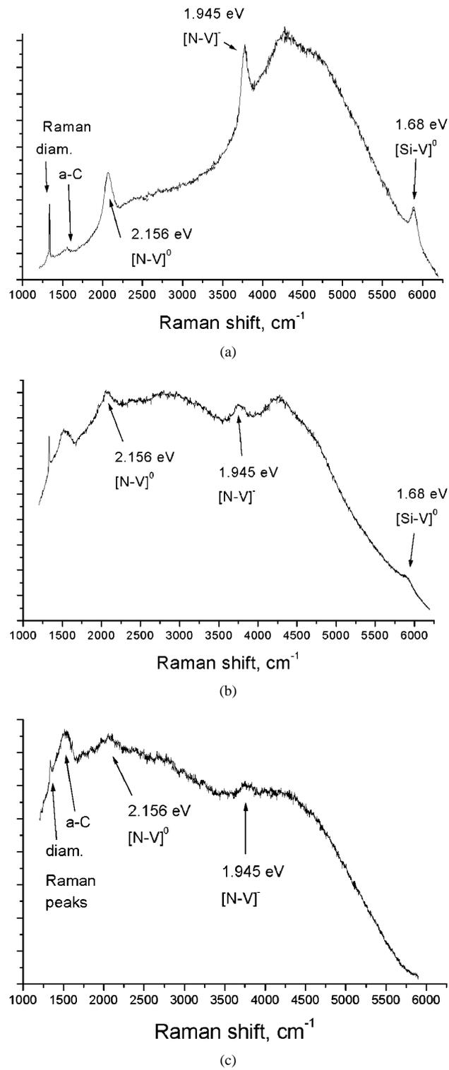
Figure 2. Room-temperature Raman and PL spectra under 2.41 eV excitation. CH<sub>4</sub> flow rate and a-C concentration in the film increases from (a) to (c).
