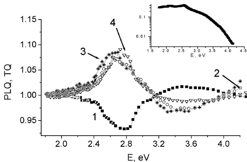
**Figure 3.** Quenching spectra of the room-temperature PL, excited at 2.4 eV, and transmittance (PLQ and TQ) for a CVD film: 1 (—■—) PLQ measured at 1.945 eV, 2 (—○—) PLQ at 2.156 eV, 3 (—◆—) PLQ and TQ at 1.68 eV, 4 (—▽—) TQ at either 1.3, 1.4, 1.5 or 1.6 eV. The inset shows the spectral dependence of the quenching source measured by a spectrally independent Golay detector.
