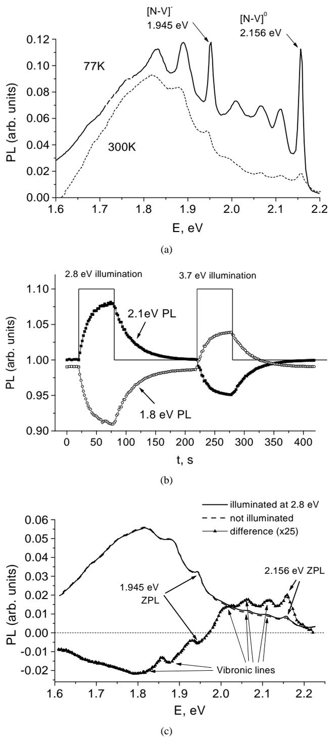
**Figure 1.** (a) PL emission from the 1.945 eV and 2.156 eV centres measured at 77 and 300 K. (b) Normalized changes in PL measured at 2.1 eV and 1.8 eV at 300 K under additional illumination with the photon energy of 2.8 eV and 3.7 eV. (c) Room-temperature PL spectra with and without 2.8 eV illumination, and the difference spectrum.
