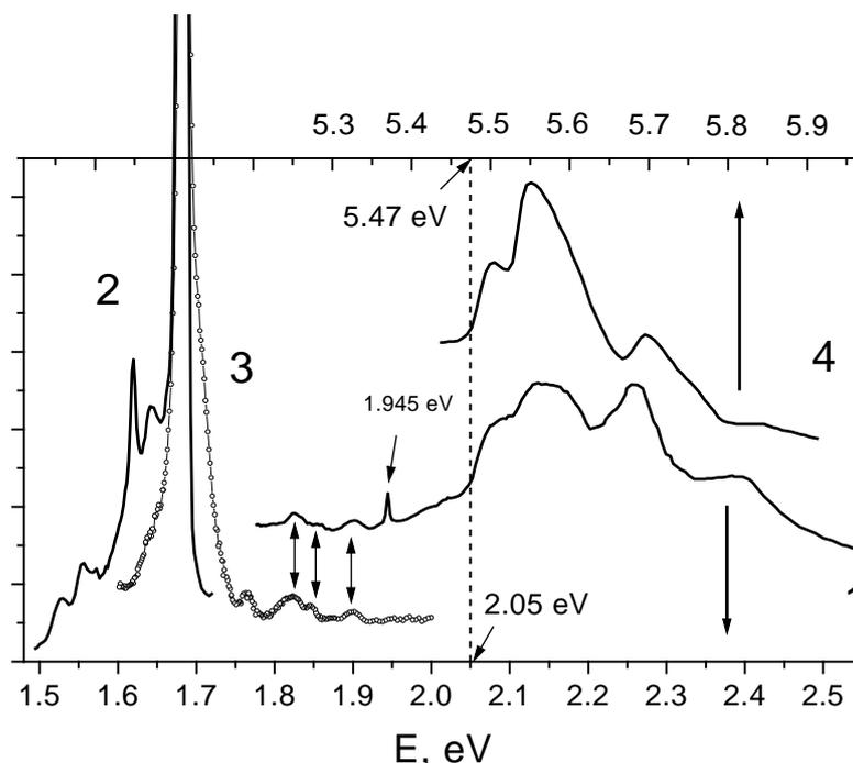
**Figure 5.** Details of the PLE spectrum from figure 4. Curve 1—PLE spectrum; curves 2 and 3—luminescence and absorption spectra of the 1.68 eV system; curve 4—PLE spectrum of the broad blue band in natural diamond in the range of intrinsic absorption (note the different  $x$ -axis) taken from data of Dean and Male (1964).
