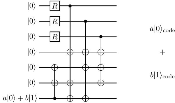
Figure 8: An encoding circuit for Steane's 7-qubit code.
