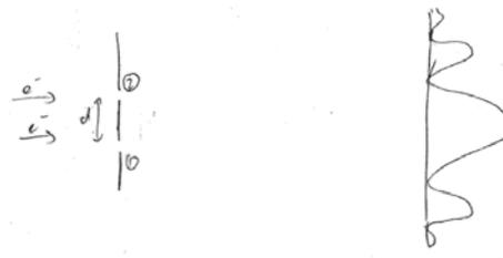
Figure VIII: Interference pattern for double slit. The interference pattern persists even if there is only one electron in the apparatus at any given time.
